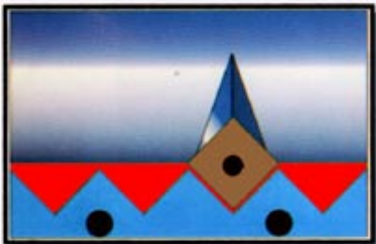
Conventional "Smooth" Rotor w/Milled-In 4-Point Cutters
