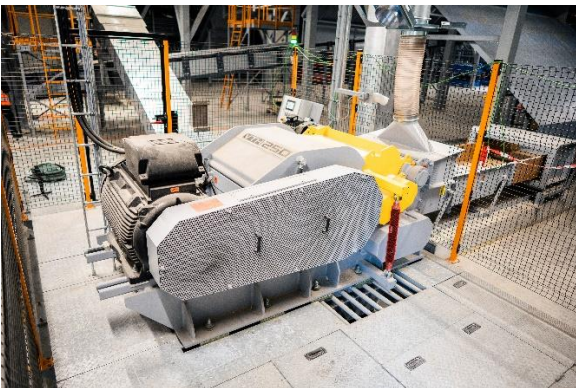
Photo 3: The drum chipper reduces the waste wood to a maximum chip length of 15 millimetres.
