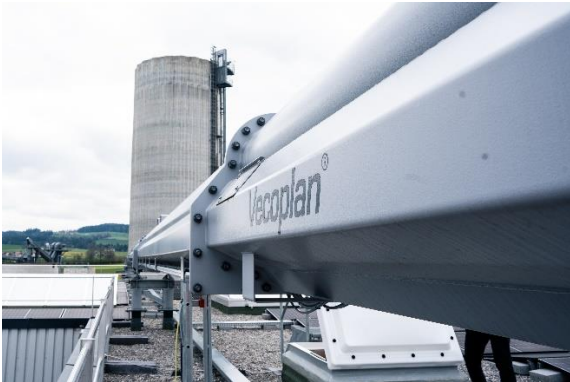
Photo 5: Outside the building, Vecoplan bottom-strand chain conveyors and pipe conveyors transport the processed material to the pellet facility in a dust-free procedure.
