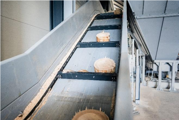
Photo 2: The conveyor system transports the pile caps to the VHZ 1600 for pre-shredding.
