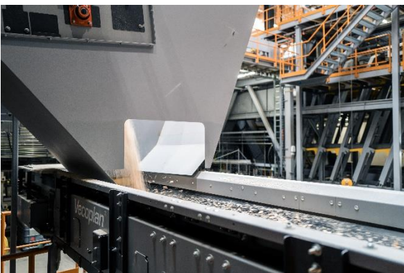
Photo 4: The conveying technology installed by Vecoplan transports the material within the disposal line, continuously and safely.
